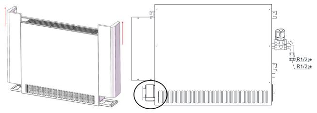
Step 2: Loosen screws on the mounting brackets. EC motor can be removed.
