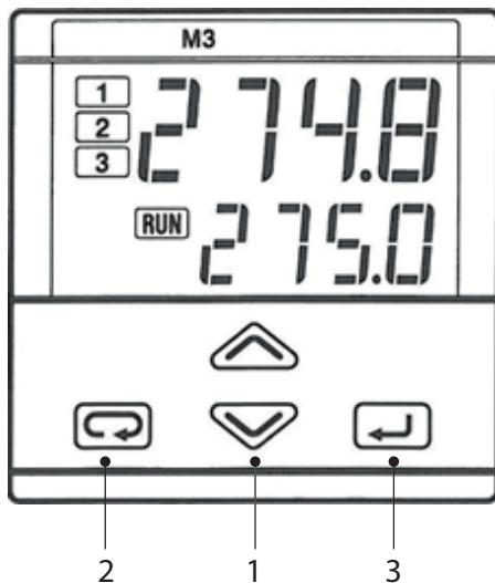
The controller displays the temperature of the water in the boiler and allows setting three thresholds on the probe working range.
