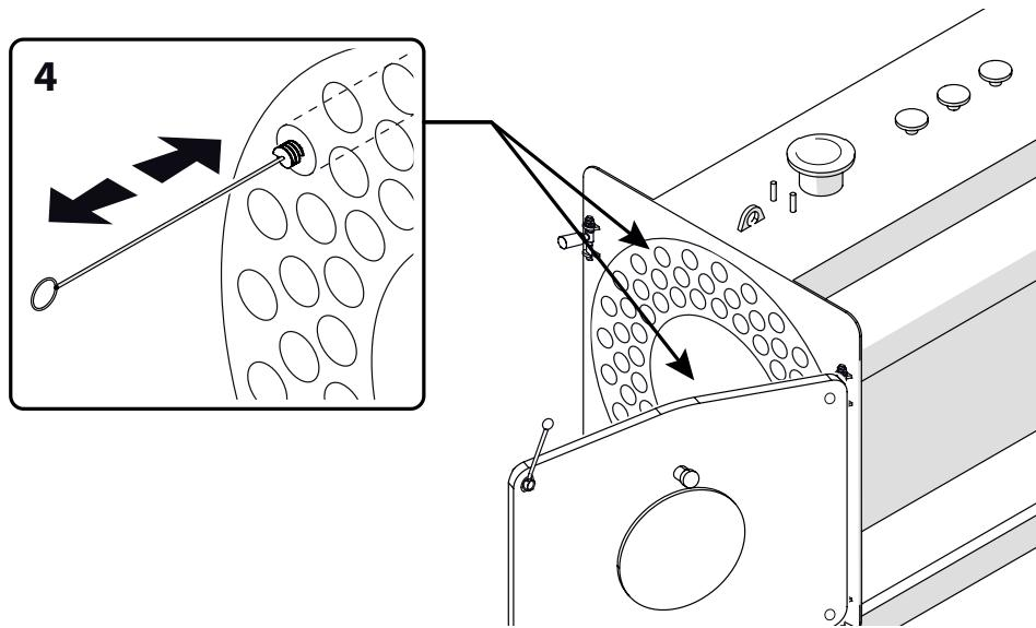
If necessary, remove the smokebox and replace the gasket before refitting it.
