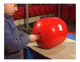
2. Once the pressure is discharged, unscrew the nuts of the blocking counter-flange and remove it;
