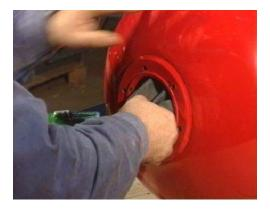
Insert the new membrane rolled up inside the tank, holding the neck of the membrane against the flange;
