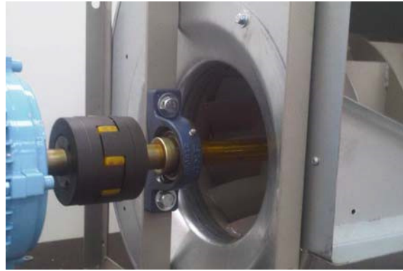
Fan with pillow block bearing
