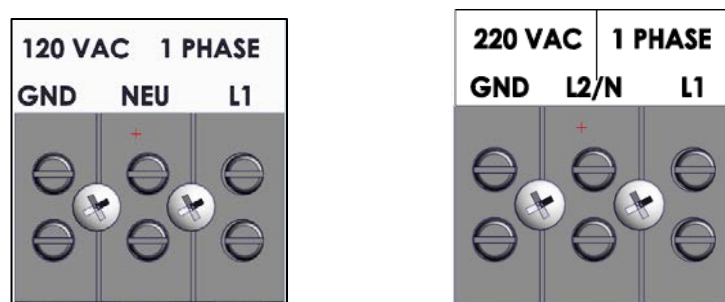
Figure 2-10. AC Terminal Block Configurations for 110 and 220 VAC Input
