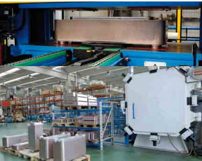
In the new fully automatic test machine the brazed plates heat exchangers are tested for a working pressure up to 30 bar (45 bar for the H version).
