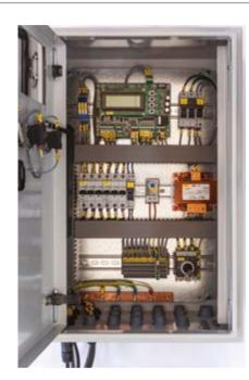
Q3E - ELECTRICAL PANEL FOR EC FANS WITH PAINT COATED METAL CASING, CONTROLLER MOUNTED INSIDE THE BOX, PROTECTED BY AUTOMATIC SWITCHES (CIRCUIT BREAKERS) CONNECTED TO GROUPS OF FANS, FAN REGULATION CONTROL MODBUS RS485, INTERNAL ANTI CONDENSATE HEATING ELEMENT
