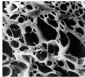
Ultra-porous microscopic structure of activated carbon
