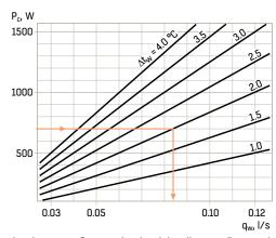
Correction for water flow, on basis of the diagram "Correction of cooling effect for water flow other than 0.05 l/s" is obtained K =  $P_{c\ 0,083}/P_{c0,05}$  = 1,05. The actual effect is therefore 5 % higher than the result given by the diagram, due to the higher water flow.  $P_c$  = 1,05 x 218 = 229 W/m
