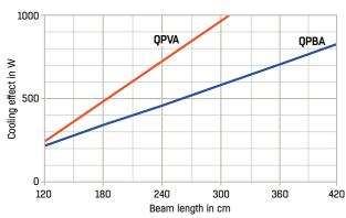
The diagram shows the approximate cooling effect,  $P_{\rm tot}$  in W with water flow,  $q_{\rm W}$  = 0.05 l/s difference between room air temperature and average water temperature = 8 °C and max sound pressure level  $L_{\rm A10}$  = 30 dB(A).
