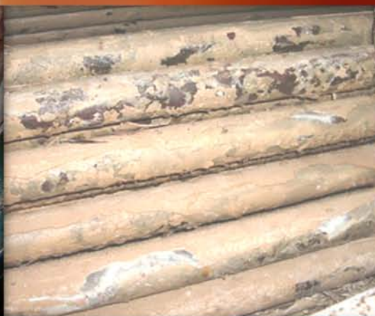
The Disintegrating Tube Surface Hard Scale
