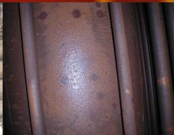
Magnetite Forms on Drum and Tube Surface
