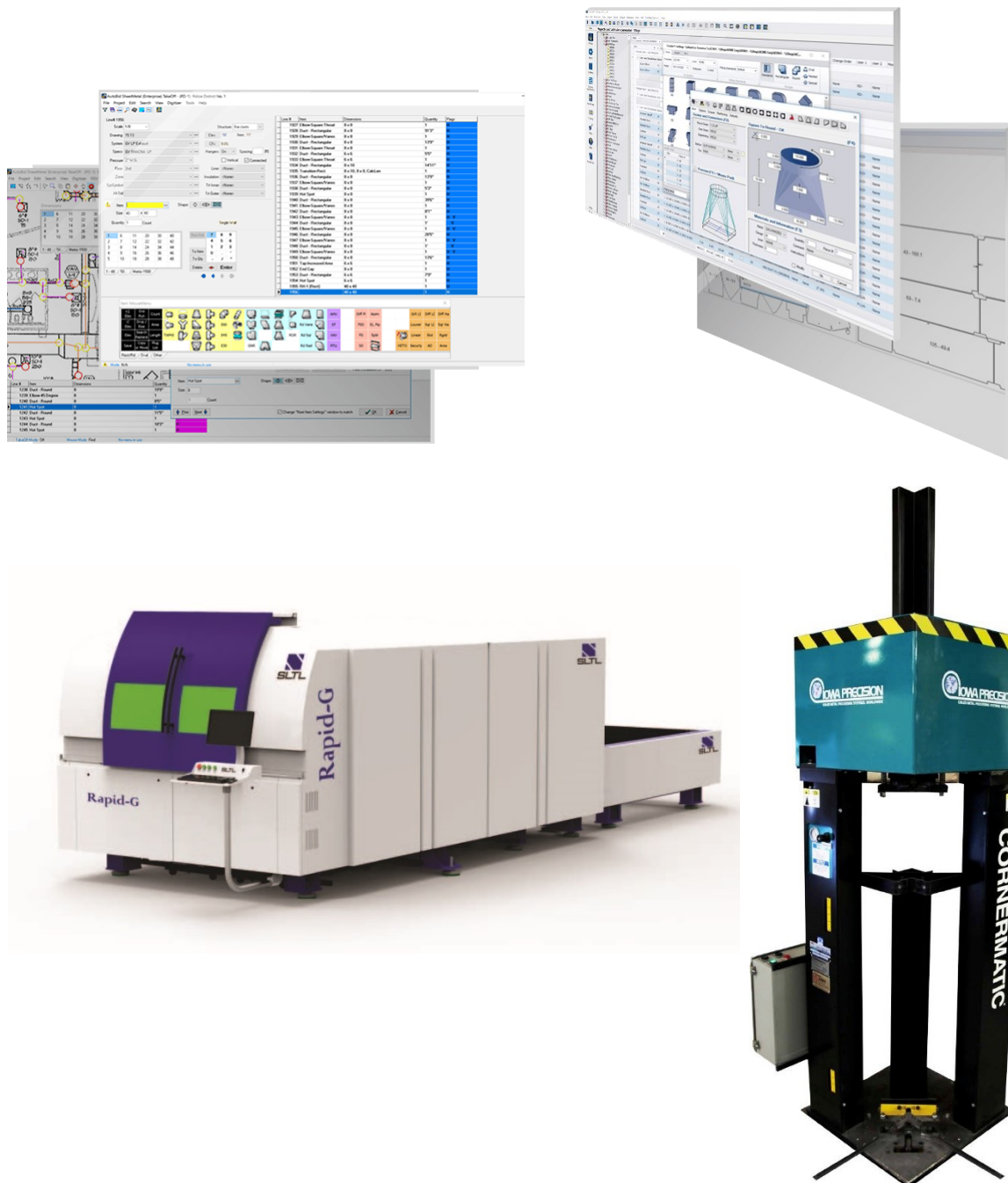
Figure 1 - The Trimble AutoBid and FabShop software drives our SLTL Rapid-G laser cutter system and automated Cornermatic flange corner insertion machines at the Cooke Industries Sheetmetal Shop. It provides automated pricing, detailing of ductwork, works out the optimum nesting of components, and automatically controls the laser-cutting unit and automated coil line for rectangular duct production.
