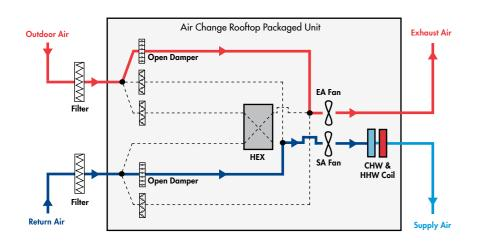
Used when 100% fresh outside air is not required (eg. when room occupancy levels are low). Outside air volume can be modulated between 0% and 100% to provide the minimum required fresh air and achieve further energy savings.
