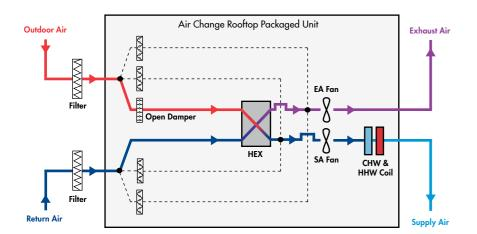
Used when the outside air temperature is hot or cold, and the indoor space requires 100% fresh outside air. The air-to-air heat / energy exchanger minimises the outside air load.
