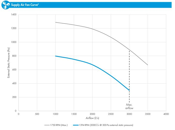
\* Fan curve makes allowance for internal pressure drop of unit (excluding filters). This pressure drop is subject to change, depending on project requirements. Supply air fan selection options are available.
