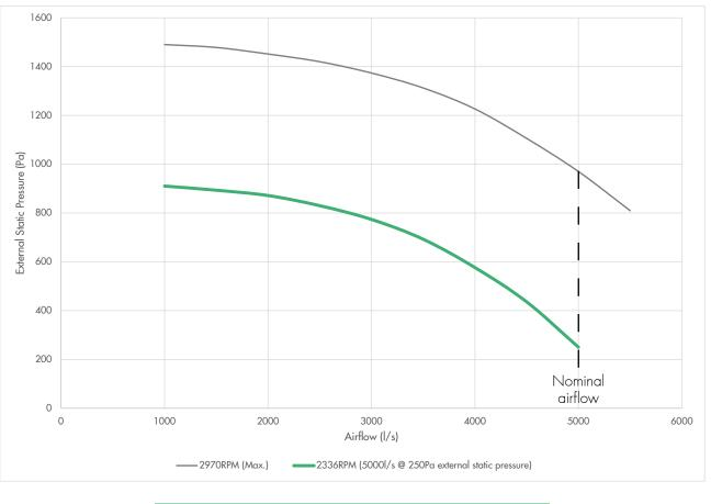
Exhaust Air Fan Power (5000l/s @ 250Pa External Static Pressure)\* Absorbed Power (all fans combined) 4.44kW
