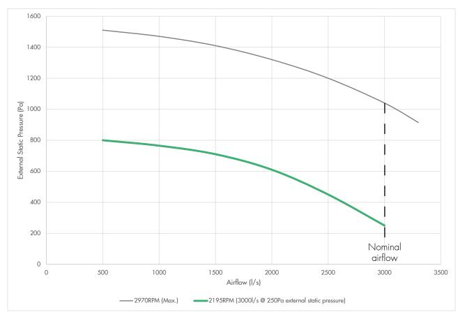
Supply Air Fan Power (3000l/s @ 250Pa External Static Pressure)\*
