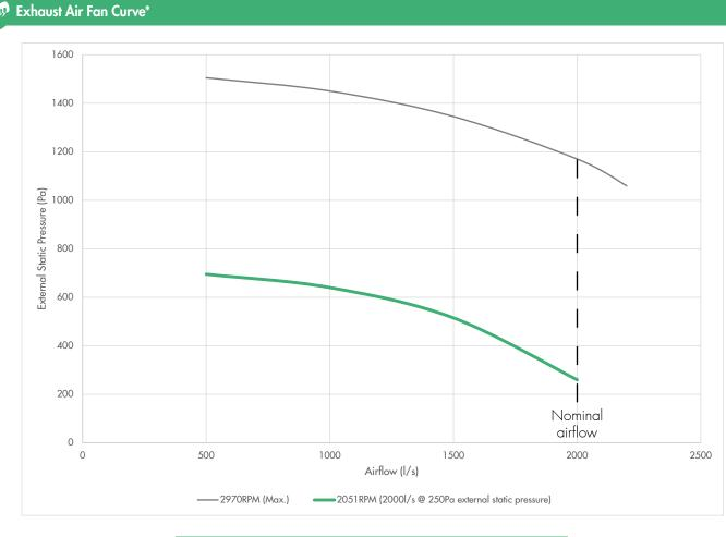
Exhaust Air Fan Power (2000l/s @ 250Pa External Static Pressure)\* Absorbed Power (all fans combined) 1.63kW
