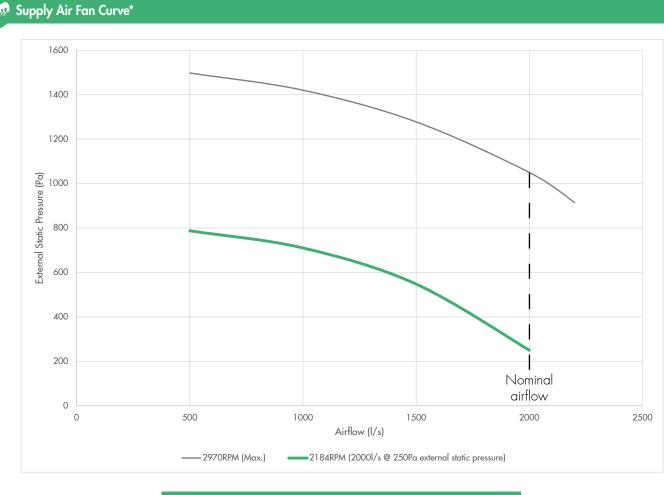
Supply Air Fan Power (2000l/s @ 250Pa External Static Pressure)\* Absorbed Power (all fans combined) 1.98kW
