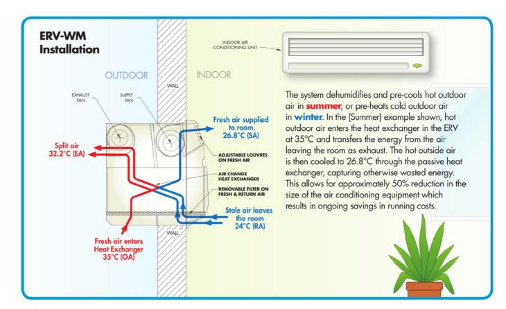
The ERV-WM unit can be located anywhere on an external wall or window of an air conditioned room, and is designed for a simple installation. Outdoor/Return air filter is accessible from inside the room.
