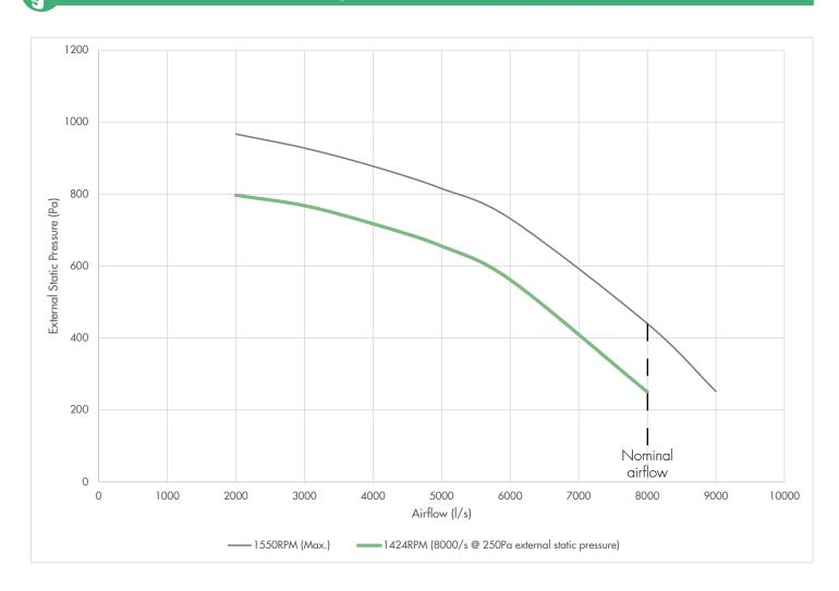
\* Fan curve makes allowance for internal pressure drop of unit. This pressure drop is subject to change, depending on project requirements. Exhaust air fan selection options are available.
