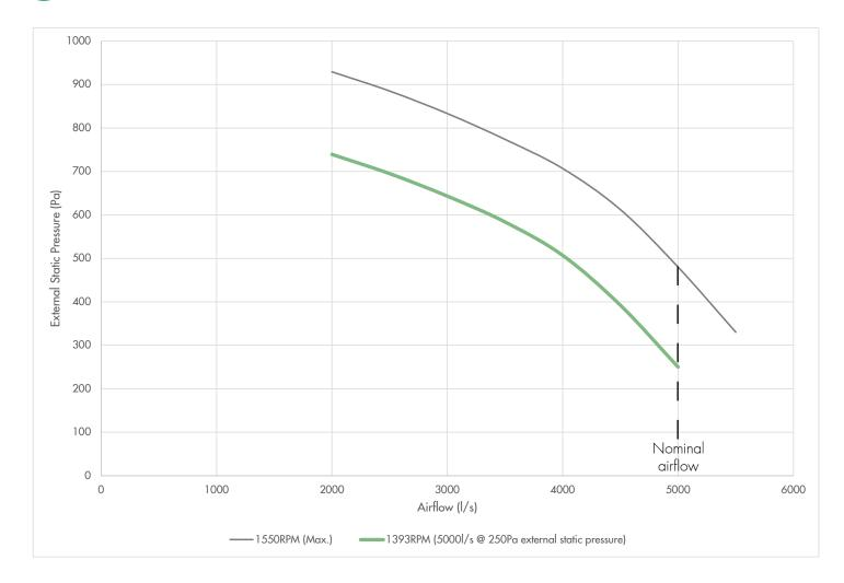
\* Fan curve makes allowance for internal pressure drop of unit. This pressure drop is subject to change, depending on project requirements. Supply air fan selection options are available.
