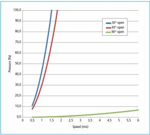
The wide open pressure drop can be calculated from the damper dynamic pressure using a K value of 0.5.
